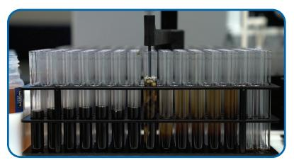
Gas infusion mixing of used oil and solvent with SampleSense Oil system just prior to analysis on Agilent 5900 ICP-OES
